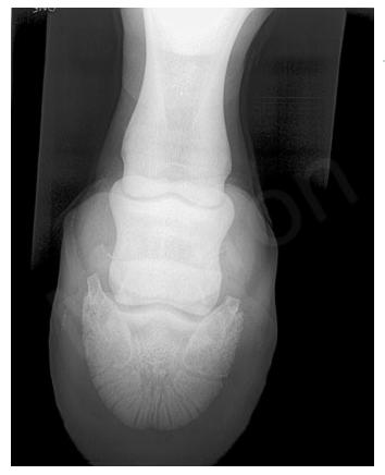
The heel effect - the outer edges of the plate appear less exposed than the center reminding us of the Inverse Square law, the outer edge of the plate is further away from the x-ray generator than the center. Also some x-ray generators will throw more energy to the right or left of center than its opposite. In most cases, this is not a big deal because the object of interest is mostly in the middle of the image.
